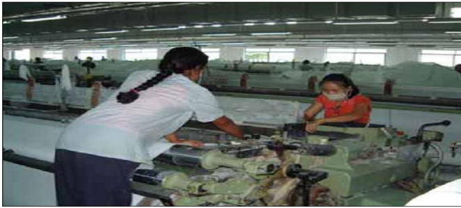
Fig. 2. Workers are performing unsafe acts by leaning over poorly guarded machines (unsafe conditions). Look at the workers clothing, hair etc.
